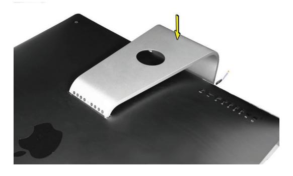
3. Remove the access card, and remove the eight T10 clutch-to-stand screws.
